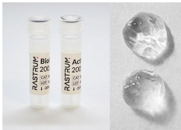
**Figure 1:** **RASTRUM** matrices are formed from a PEG-based bioink that instantly gels at room temperature when combined with an activator solution. The matrices are biocompatible, transparent hydrogels that can be modified to suit the cell type.
